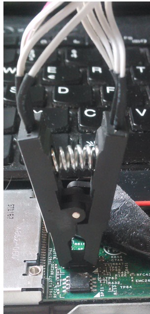
Figure 13: Clamp to program EEPROMs without the necessity to solder them to a programming pad first
